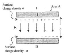
For uniform electric field, potential difference is simply the electric field times the distance between the plates. Capacitance of parallel plate capacitor is , the charge required supplied to either of the conductors of the capacitor so as to increase the potential difference by unit amount.
